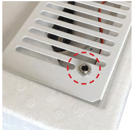
Figure 6. Two 12V outputs for LED lightning are placed on top front of e-Coolio.
